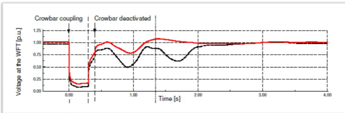
Figure 6. Voltage at the wind farm terminal
