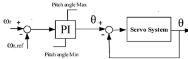
Figure 3. Pitch angle controller
