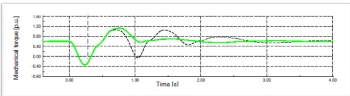
Figure 10. Torque fluctuations of the fixed speed induction generator
