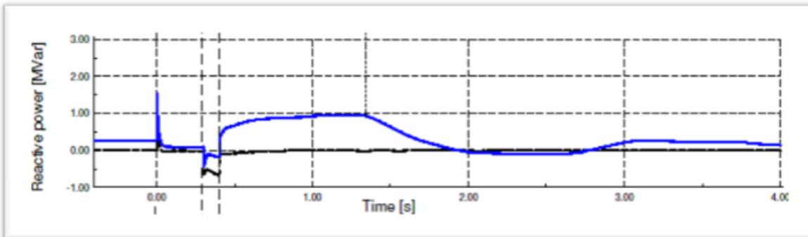
Figure 8. Reactive power output of the wind farm
