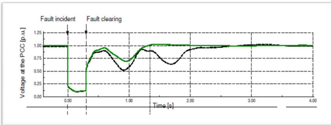
Figure 5. Voltage at the point of common coupling
