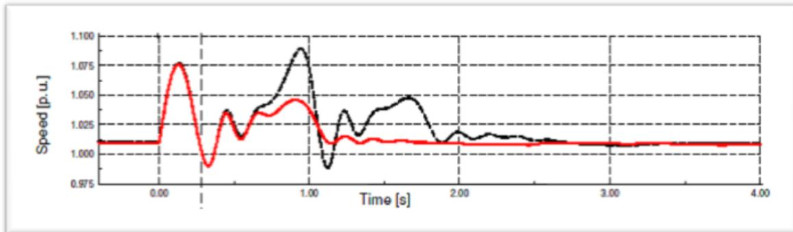
Figure 9. Speed of the fixed speed induction generator
