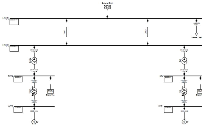
Figure 4. Wind farm grid connection model
