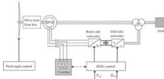
Figure 1. Arrangement of the doubly fed induction generator wind turbine concept
