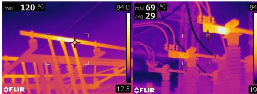
Fig.3. 11KV Busbar Assessment
