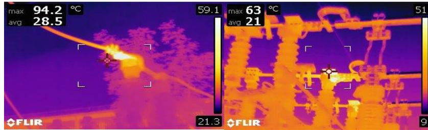
Fig.5. Cable/overhead jumper on pylon Assessment
