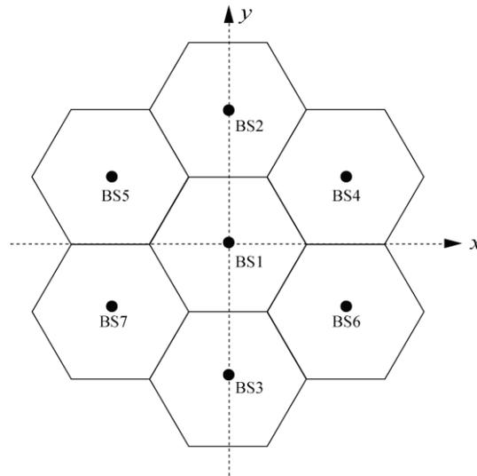
Figure 1. Seven-cell system layout.
