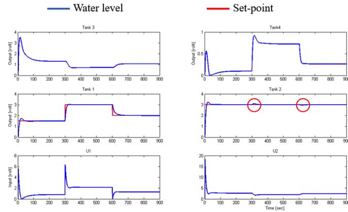
Figure 3: Simulation response of the QTP (minimum phase characteristics) with a Decentralised SISO PI Controller
