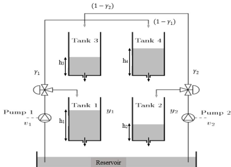
**Figure 1.** Schematic Diagram of the Quadruple Tank Process
