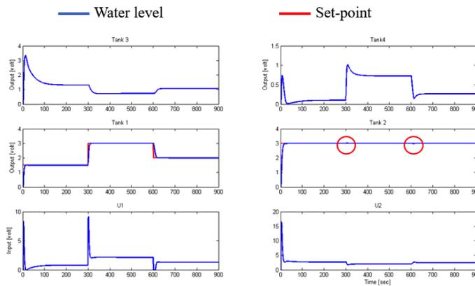
Figure 4: Simulation response of the QTP (minimum phase characteristics) with a Decentralised SISO LQ-PIP Controller
