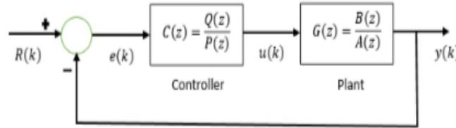
Figure 2: Block diagram for the Design of PI Controller
