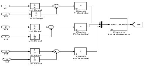
Fig. 9. Shunt controller with PID controller for UPQC
