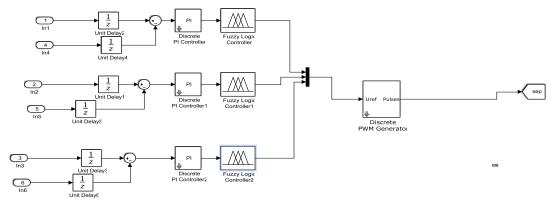
Fig. 10. Shunt controller with fuzzy logic controller for UPQC
