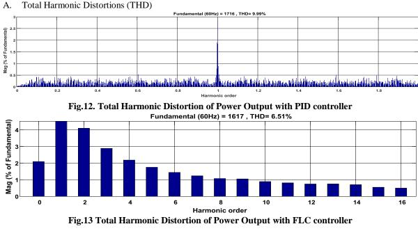
Fig. 12 and 13 shows Total Harmonic Distortion of output voltage of proposed system with UPQC with implementation of PID and FLC respectively. These results shows that while using PID there is distortion of 9.99 % in output while with FLC the system output has 6.51% THD.
