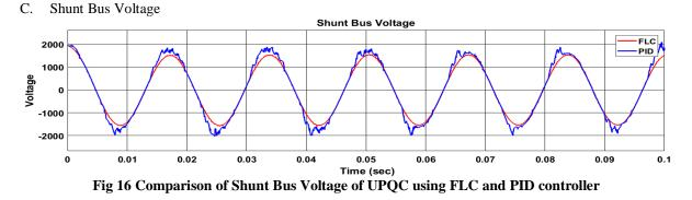
Fig. 16 shows shunt controller bus voltage of proposed system with UPQC with implementation of PID and FLC respectively. These results shows that while using PID there is distortion in output while with FLC the system output is stable and constant.
