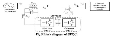
In industries and domestic usage, we are having large numbers of single phase loads which employs solid state control which requires the attention to the problem of harmonics occurring due to its usage. These solid state controllers try to convert and also control ac power fed to many loads and thereby increase efficiency of the system and in this process they also introduce harmonic components in the lines which create several problems which need to be solved.
