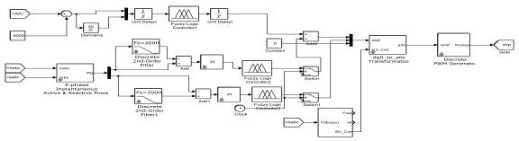
Fig. 11 Series controller with fuzzy logic controller for UPQC
