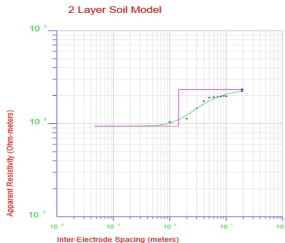
**Fig. 9.** Two-layer soil modelling result
