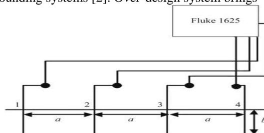
Fig. 1. Wenner 4-pole method can be used to measure earth resistance of a given location for homogeneous soil environment
