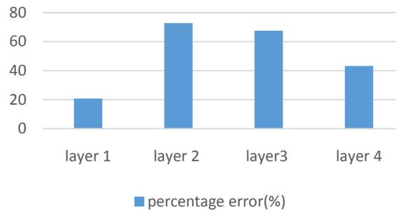
Fig. 14. Percentage error between thickness obtained from RESAP and Bore-hole
