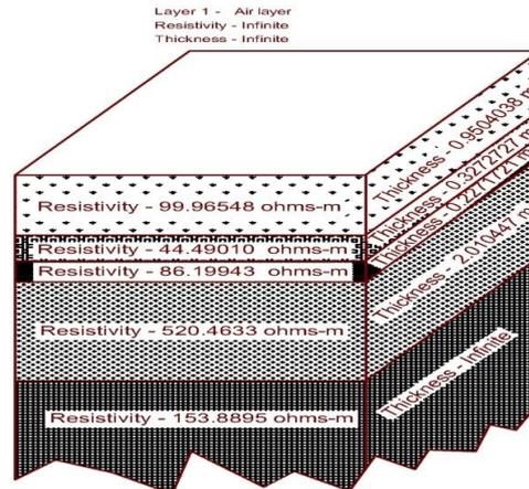
Fig. 13. Five-layer soil modelling 3D representation
