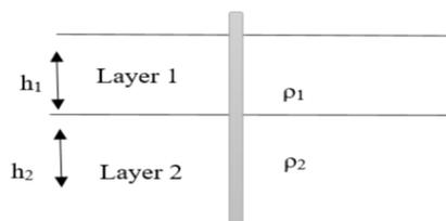
Fig. 3. Two-layer soil model
