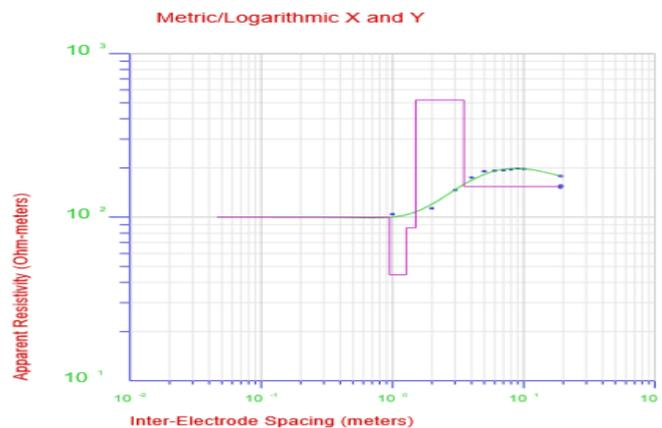
Fig.12. Five-layer soil modelling result
