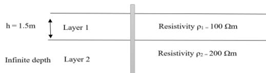
Fig.8. Two-layer soil model
