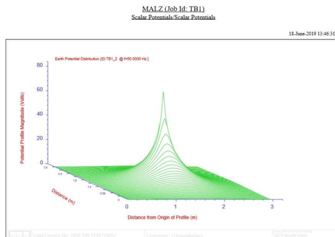
Fig. 17. 3D map of surface voltage profile distribution
