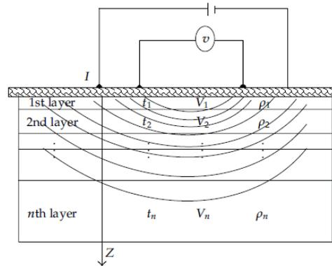
Fig. 4. Multi-layer soil model
