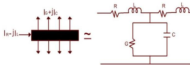
Fig. 2. Current components in the soil
