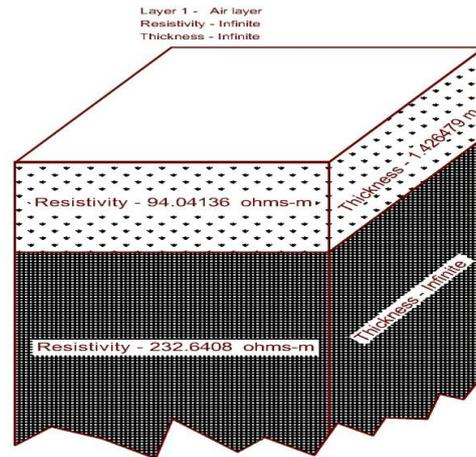
Fig.10. Two-layer soil modelling 3D representation
