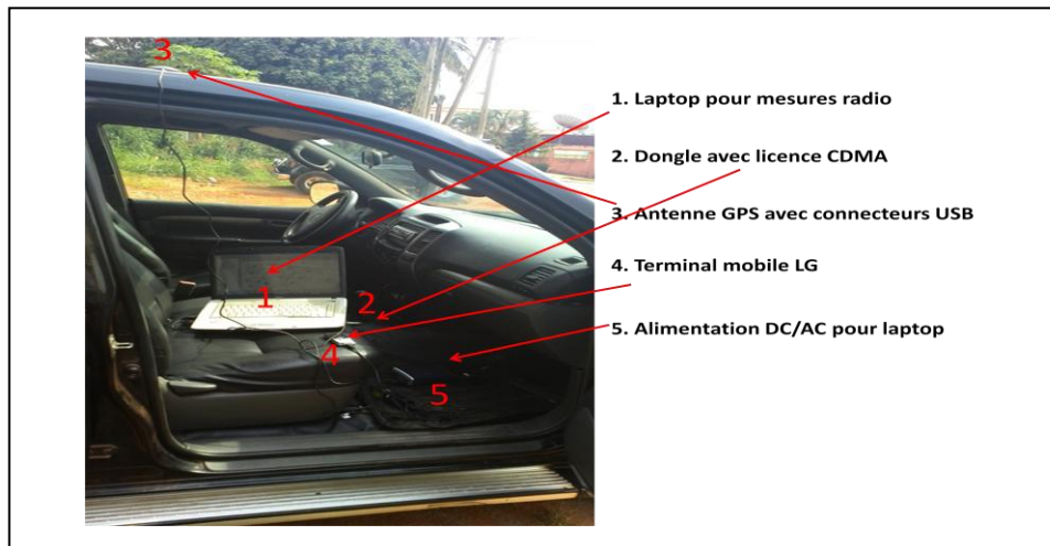
Figure 1: Drive test measurement kit installed on vehicle.
