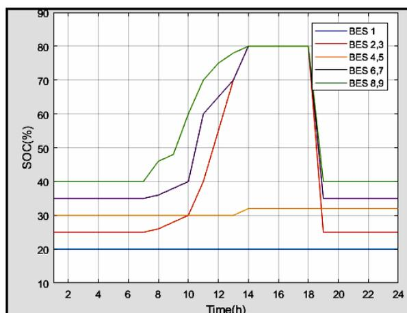
Figure 5 SOC Variation of charging and Discharging
