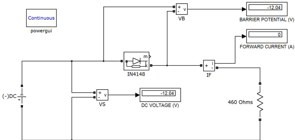
Fig 2.c.Circuit arrangement of reverse bias
