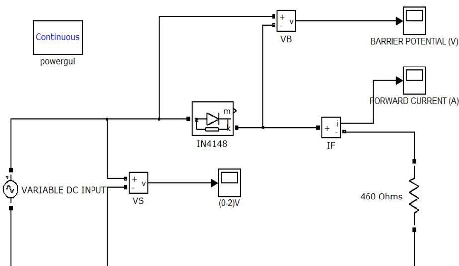
**Fig 1.a.**Forward bias circuit arrangement
