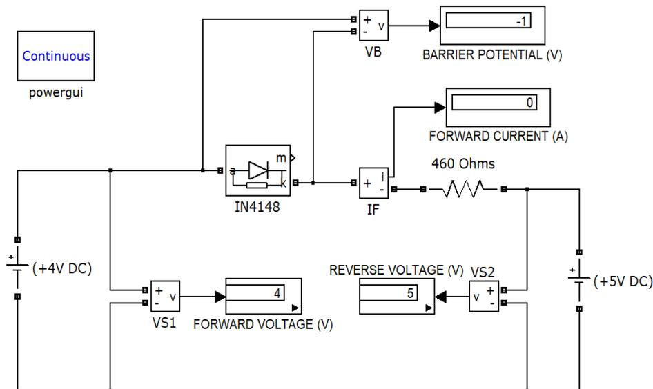
Fig 4.a.Reverse bias circuit arrangement with two dc supply
