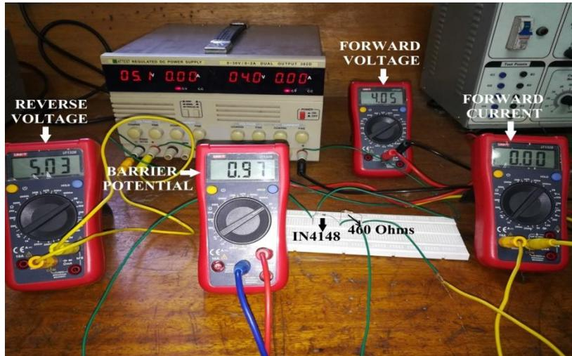
Fig 4.b.Reverse bias experiment with two dc supply
