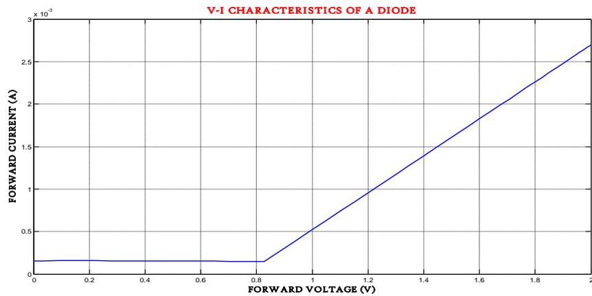
Fig 1.e.Forward voltage and current characteristics of diode
