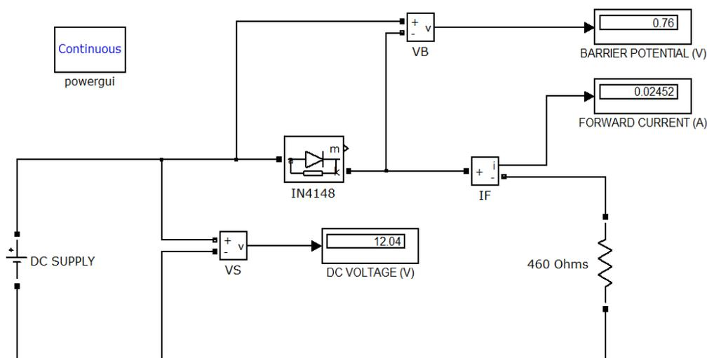
**Fig 2.a** Forward bias with fixed dc input voltage
