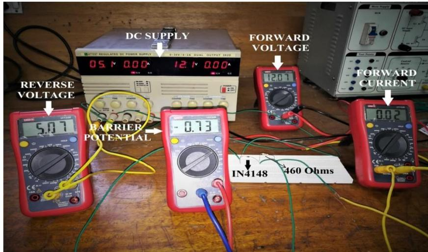
Fig 3.b.Forward bias experiment with two dc supply
