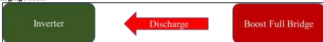
Fig. 3 Schematic of power interface in Discharging mode [2]
