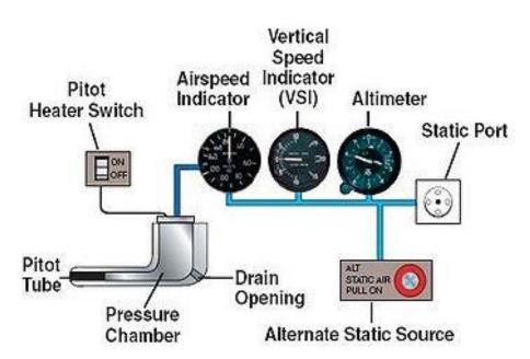
The pressure all meter. a simple, reliable pressure gauge calabrated to indicate height, the pressure at a the weight of the Column of air o paint depends on Vertically upwards from the point to the cuter Limit which extends of the onmosphere, the higher a the an aircraft is flying, shorter the Column is, of air above it and Consequently the Lower is the the the pressure at the pressure, and by measuring the pressure the altimeter height.
