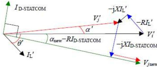
Figure 3 : phasor diagram voltages and currents
