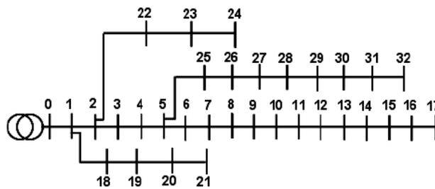
Figure 4: single line diagram of 33-bus distribution system.
