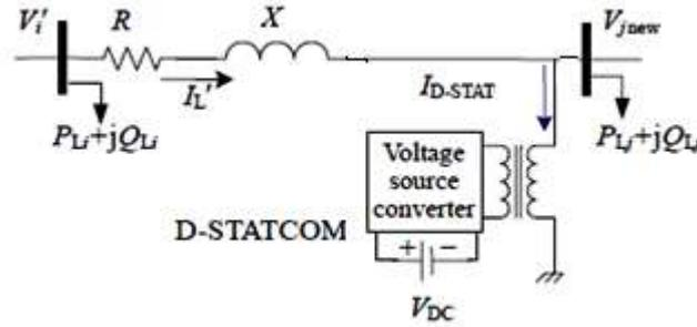
Figure 2: single line diagram of two buses with DSTATCOM
