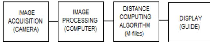
Fig. 1. Block diagram of design and implementation of dynamic distance sensor.
