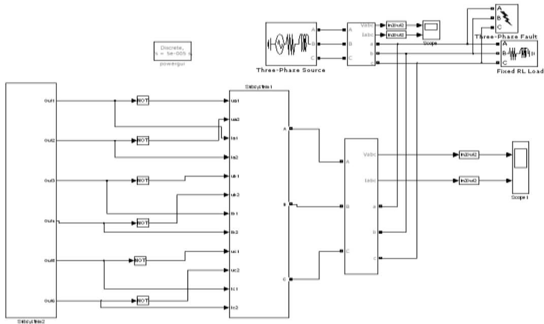
Fig (9): SPWM simulation circuit for 3-level multi-inverter
