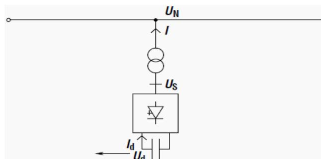
Fig (3): Schematic diagram of STATCOM
