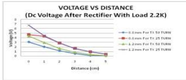
Fig 7: Output Voltage versus Distance DC Voltage after rectifier with load 2.2K resistor.
