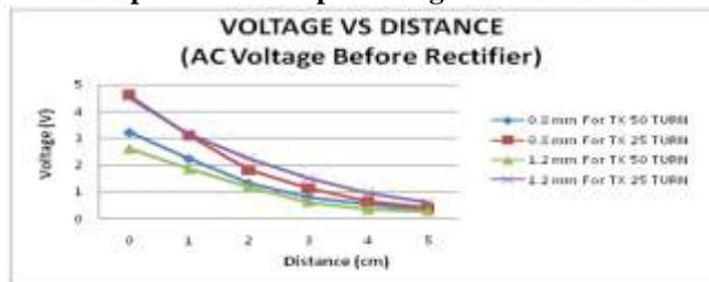
Fig 5: Output Voltage versus Distance AC Voltage before rectifier.
