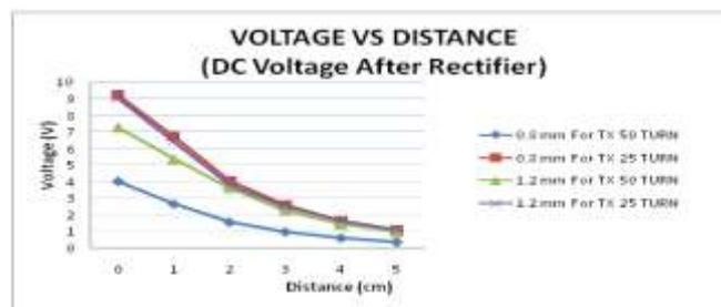
Fig 6: Output Voltage versus Distance DC Voltage after rectifier.
