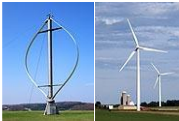
Figure (4): Two main kinds of wind turbines.
