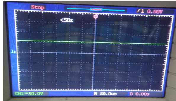
Fig 6.3 R-load's DC output voltage Vin=15V Vo=55V
