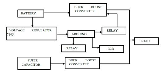
This paper hierarchical control system for the components within the islanded DC micro grid aims to optimize energy management, enhance system stability, and ensure efficient operation under varying conditions. At the core of the system lies an Arduino microcontroller unit (MCU) programmed to oversee the hierarchical control architecture. The MCU acts as the central supervisory controller, orchestrating the interaction between the various components to achieve optimal system performance.
