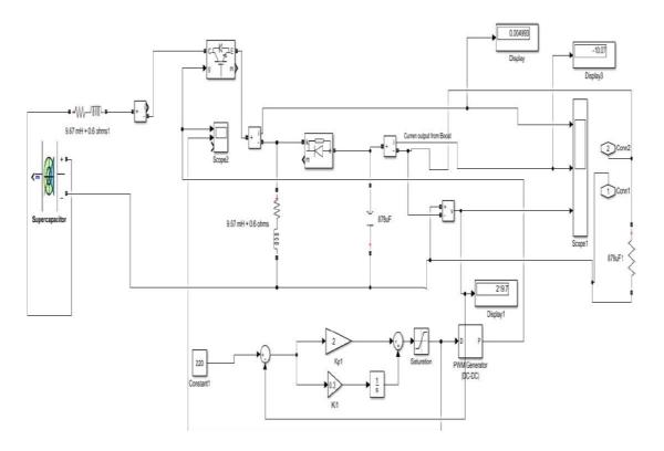
The Subsystem 2 is battery source that connected with fly back buck-boost converter. From battery side the voltage 100v and reference voltage 200v, as per load demand the converter buck or boost the voltage, the display shows normal current, boosted voltage and current through voltage and current measurement.
