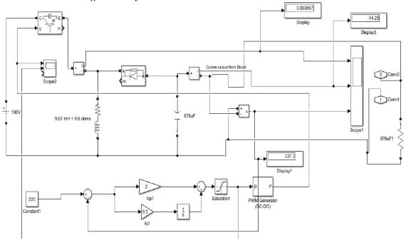
In this paper the Simulation circuit diagram it consists of two subsystem both are connected in parallel that consider as islanded dc micro grid which connected with two loads (load, load1). The load 1 work after 3sec that set-in step. The breaker is connected with load for protection from overvoltage. A simulation is a model that mimics the operation of an existing or proposed system, providing evidence for decision-making by being able to test different scenarios or process changes.
