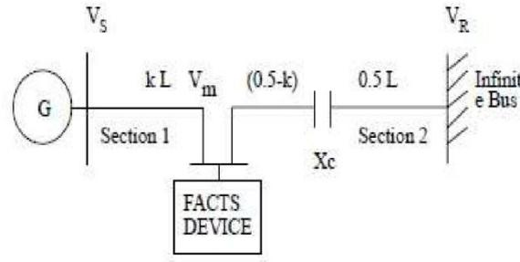
Fig 3. 2-Port, 4-terminal model of a transmission line
