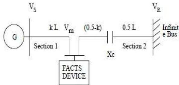
Fig 4. Series compensated transmission line with a shunt FACT device [3].
