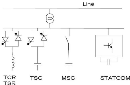
Fig 6. Examples of FACTS for shunt compensation.
