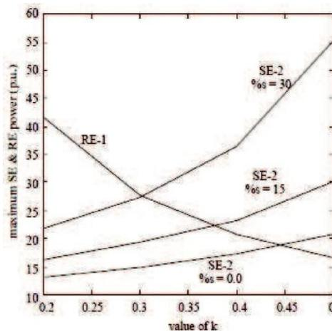
Fig 10. Variation in the maximum RE power of section-1 and SE power of section-2 against k for diff. value of %S.
