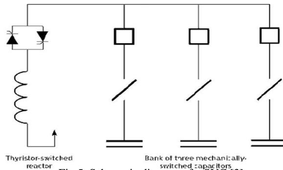
Fig 5. Schematic diagram of a SVC [3].
