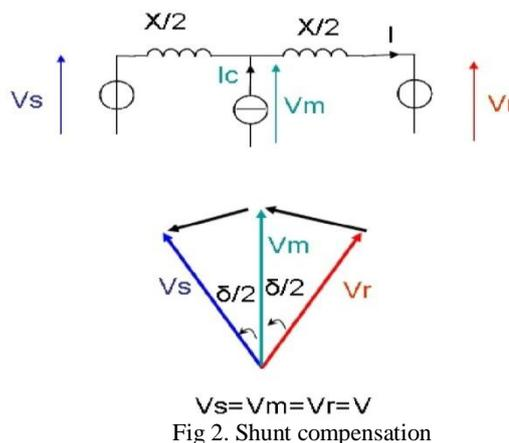
Fig 2. Shunt compensation
