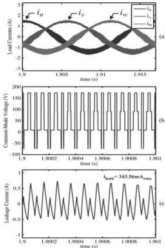
**Fig. 9. Simulation of the PV transformerless ZSI modulated by SVPWM with MCB control connected to a RL load. (a) Load currents. (b) CMV  $v_{CM}$ . (c) Leakage current  $I_{leak}$ .**
