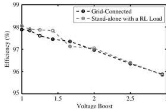
Fig.10. Simulation result of grid-connected and stand-alone ZSI-D efficiency versus voltage boost for a fixed output active power).
