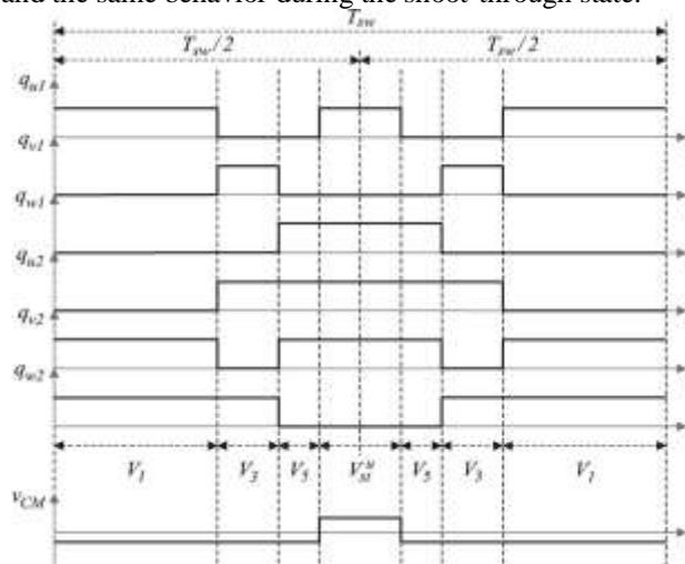
**Fig. 5. Switching pattern and CMV in the ZSI-D controlled by OPWM .**
