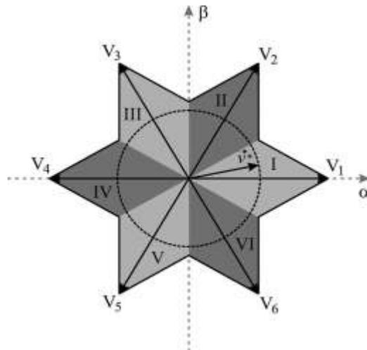
**Fig. 6. Output voltage space vectors for OEPWM in the three-phase ZSI-D.**
