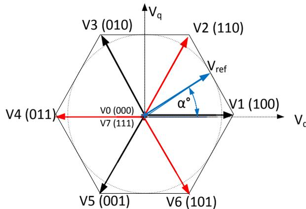
Fig. 4. Output voltage space vectors of a three-phase inverter.
