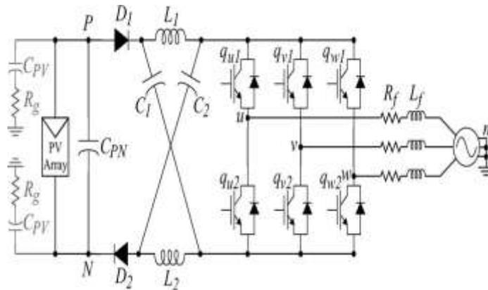
Fig. 2. Three-phase ZSI-D to reduce leakage currents in transformer less grid connected PV systems.
