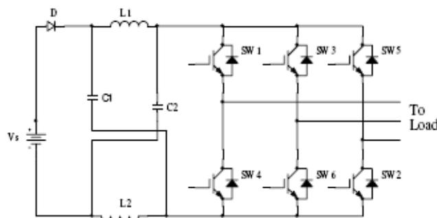
Fig.1. Z-Source inverter
