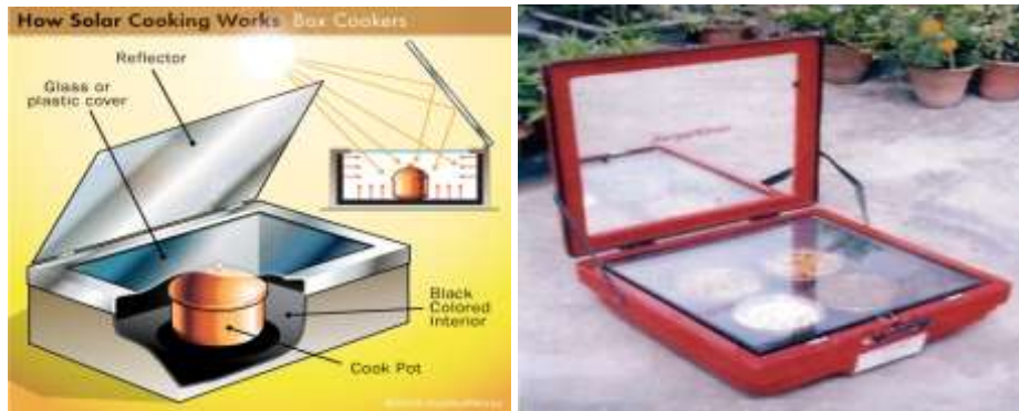
Fig.12 Solar box cooker with adjustable reflector and absorber plate
