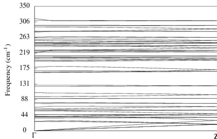
Fig. 9: The Phonon spectra of  $PbSnS_3$  along  $\Gamma$ -Z direction
