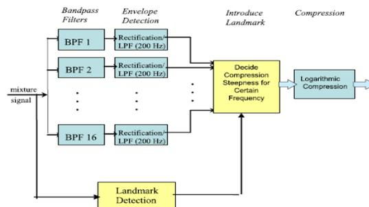
Figure 1.3 System diagram of introducing the landmark cues to the CI system panel. As can be seen from this panel, the envelopes are attenuated relative to the envelopes in the voiced segments, thereby rendering the vowel/consonant boundaries (present in the low frequencies, i.e., < 1000 Hz) more clear.
