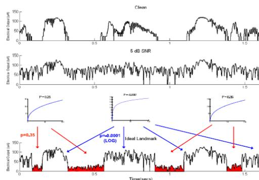
Figure 1.2 Envelope (4<sup>th</sup> channel with center frequency of 600 Hz) of clean (upper panel) signal, envelope in 5 dB SSN (middle panel) with log compression function and envelope processed (bottom panel) with varied compression steepness ( $q = -0.0001$  for unvoiced segment and  $q = 0.35$  for voiced segments).
