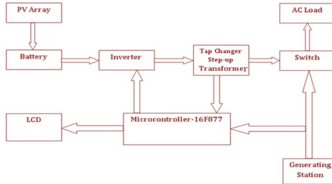
Figure 1: The block diagram of synchronization of Photo-voltaic system with a Grid
