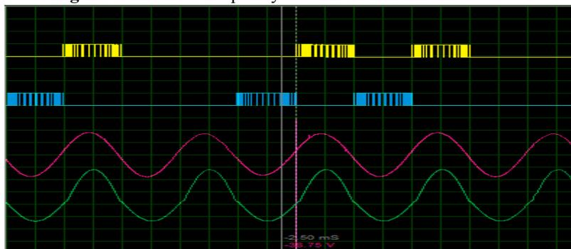
**Figure 7:** Shows the results when harmonics are eliminated by PWM
