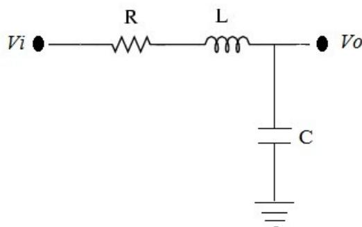
Figure 2: RLC low-pass filter
