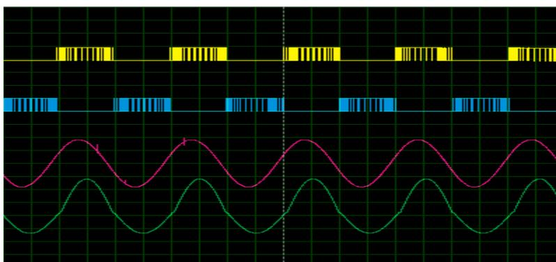
**Figure 5:** Reference system frequency changed to 48 Hz. Yellow and Blue shows operation of PWM
