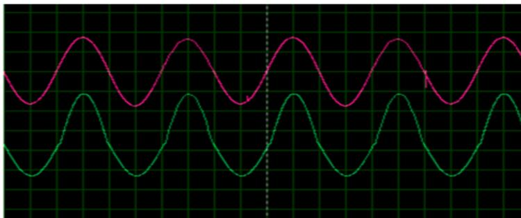
**Figure 4:** The frequency of generating system (Green) and Photo-voltaic inverted system (pink)
