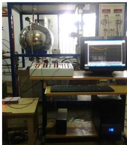
Fig 5. Real time setup of Spherical tank level process
