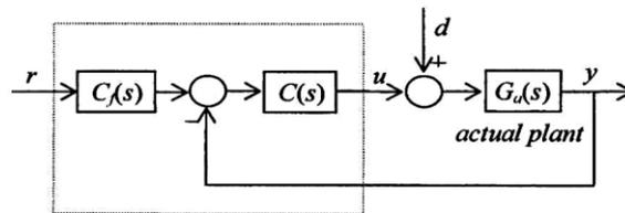
Fig. 1. A 2DOF control system structure.
