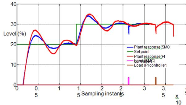
Fig 10. Comparison of plant responses with SMC-CDM and PI controllers
