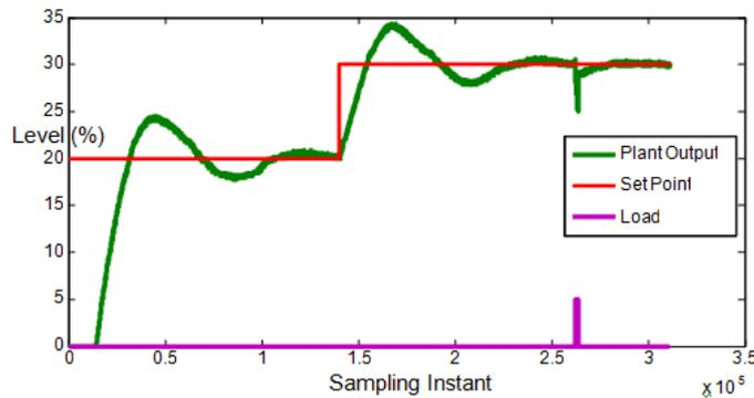
Fig 7. Servo and regulatory responses of plant with SMC-CDM controller in real time
