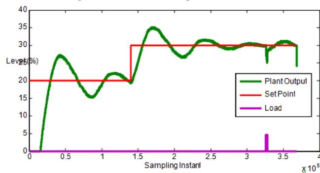
Fig 9. Servo and regulatory response of plant with PI controller in real time
