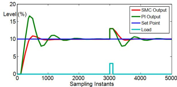
Fig 4. Comparison of servo and regulatory responses with SMC-CDM and PI controller
