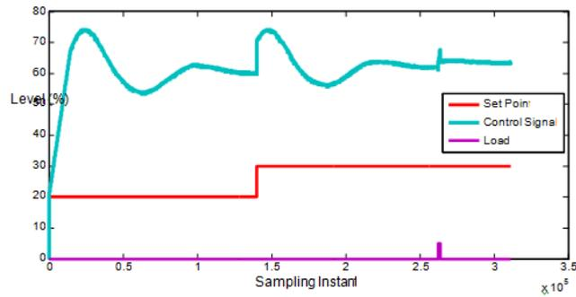
Fig 6. SMC-CDM Controller output in real time
