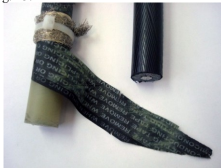
Figure 13 – XLPE cables (aged on the left and new on the right).
