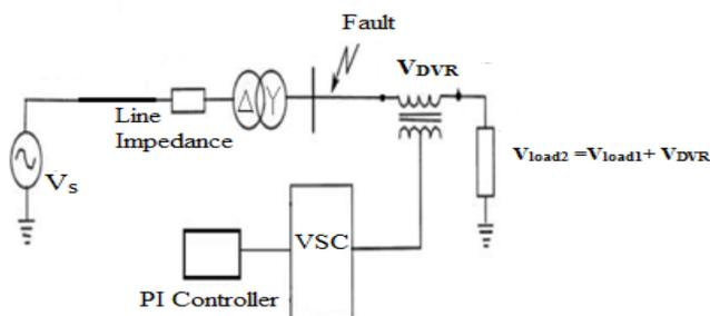
Fig.3. Overall diagram of DVR
