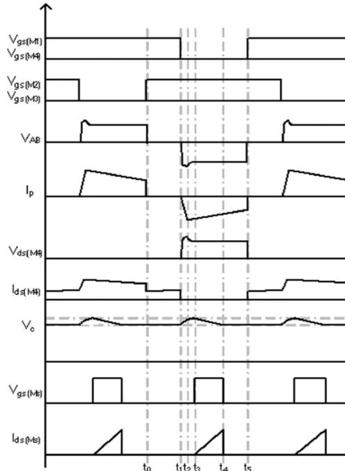
Figure 4. Operation Waveforms of Step Up Conversion
