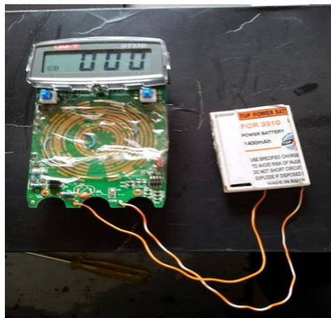
Fig (2) new designed electronic circuit connected to the Li-ion battery to Measure the potential.
