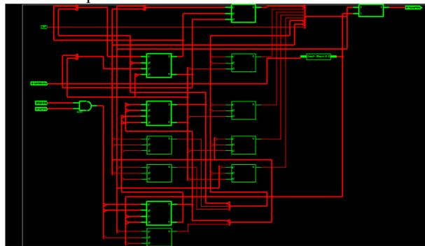
Figure 13 RTL View of 16 bit Kogge stone adder
