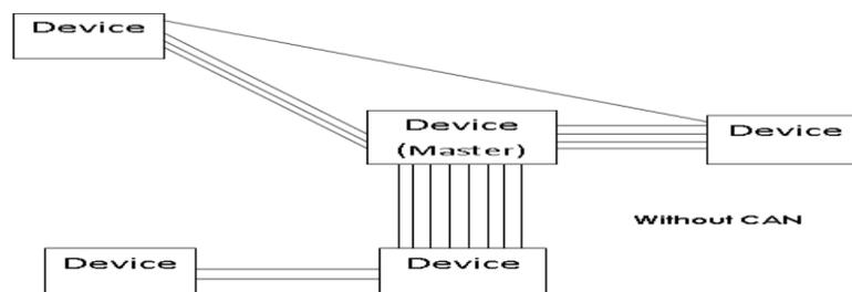
Fig. 2 (a) Traditional Wiring
