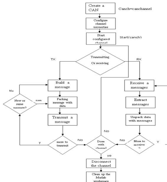
Fig. 2 Basic CAN workflow in VNT
