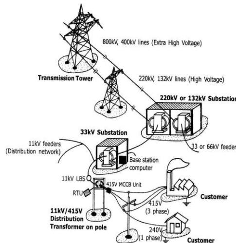
Fig. 1 Basic Distribution Structure
