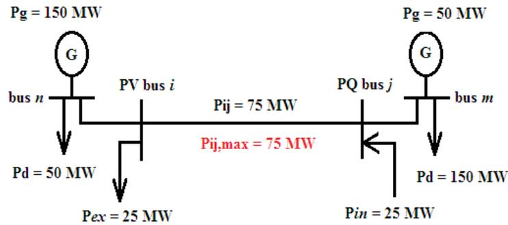
Fig. 3. Decoupled PIM of UPFC in transmission line.
