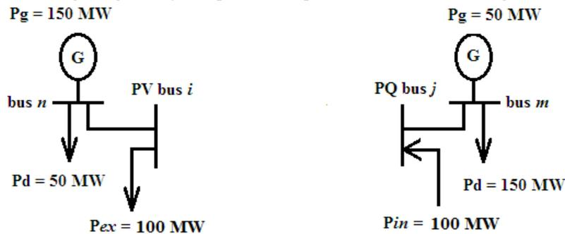
Fig. 4. Decoupled model of UPFC.
