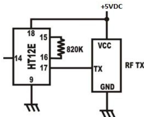
Fig. 3. RF Transmitter with Encoder
