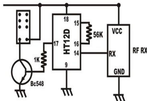
Fig. 4. RF Receiver with Decoder
