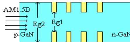
Fig. 2 Energy band diagram of GaN/InGaN MQW solar cell
