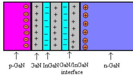
Fig. 1 Piezoelectric field in GaN/InGaN MQW solar cell structure
