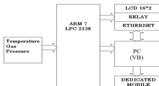
Fig.1-Remote Monitoring & Control of Industrial Parameters through Embedded Web Server & GSM Mobile
