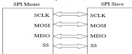
Fig.3-Serial Peripheral Interface[3]
