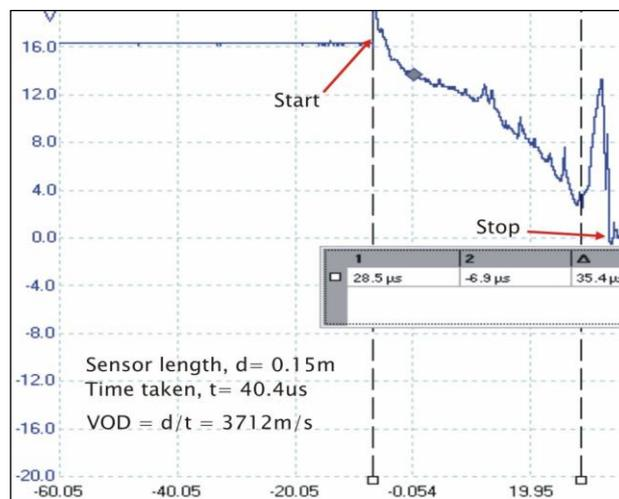
Fig.4 Voltage-Time ( $\mu$ s) graph to calculate VOD
