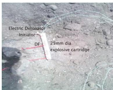
Fig. 2 D'atriche method in field Fig. 2 D'atriche method in field
