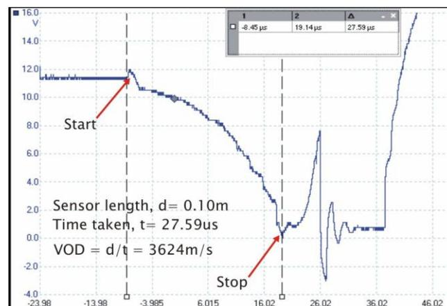
Fig.6 VOD record of SMD sensor in cartridge emulsion explosive 25mm paper tube type with double track.
