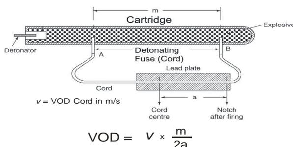
Fig. 1 D'atriche method Schematic
