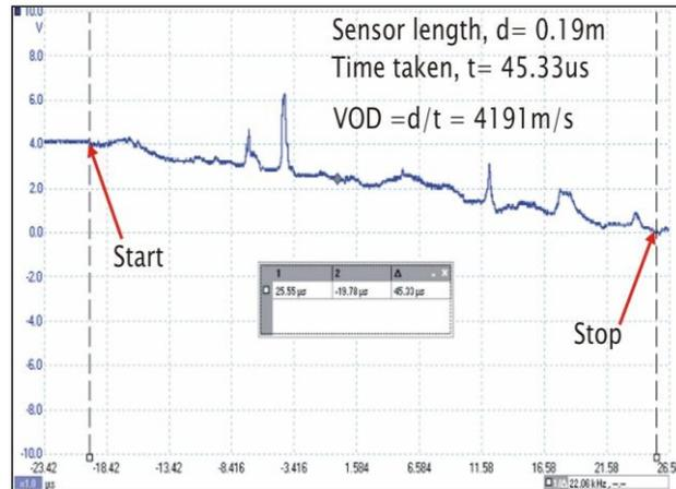
Fig.2 Voltage-Time ( $\mu$ s) graph to calculate VOD
