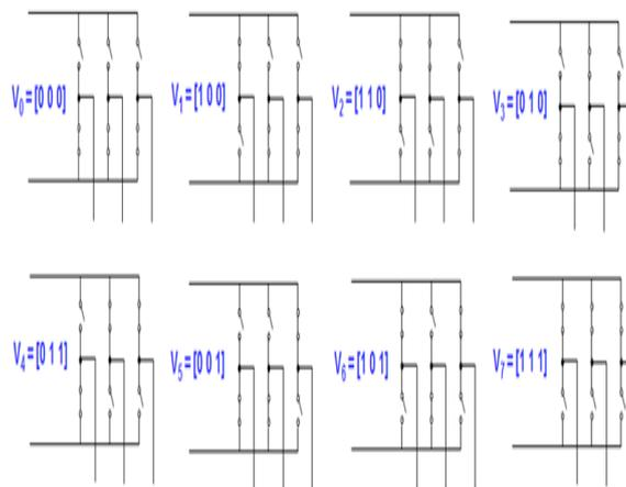
Fig6. Eight Inverter Voltage Vectors (V0 to V7)
