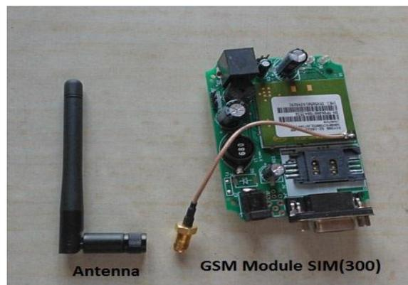
Figure 3: GSM Module sim (300)
