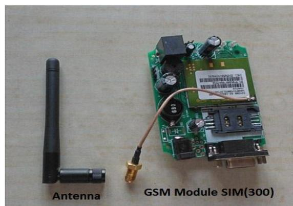
Figure 3: GSM Module sim (300)
