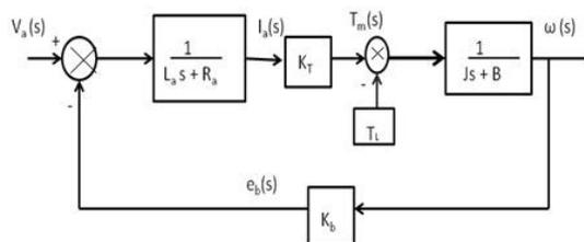
**Fig.3** Block diagram of armature controlled S.E.DC motor
