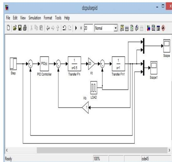
**Fig 6.** Simulink model of S.E.DC motor with PID controller
