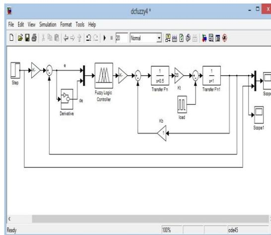
**Fig. 11** Simulink model of S.E.DC motor with Fuzzy logic controller
