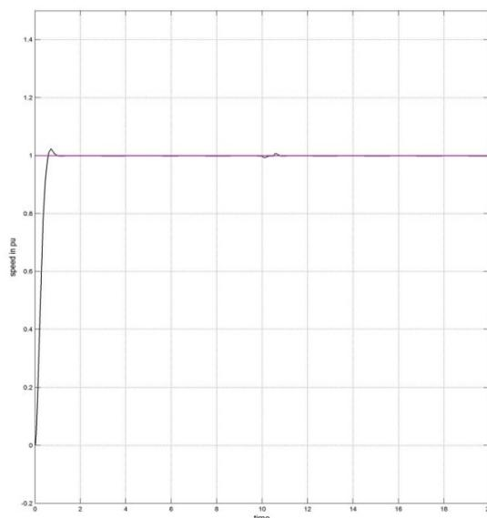
**Fig 13.** Speed response of SEDC motor with fuzzy logic controller
