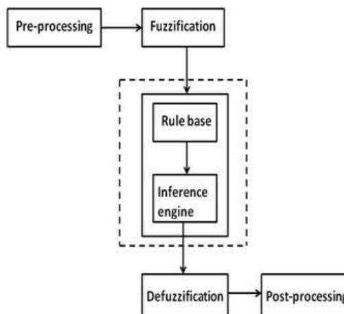
**Fig 7.** Block diagram of Fuzzy logic controller
