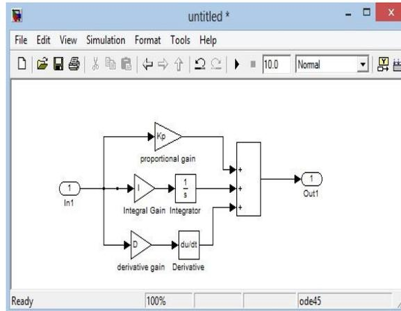
**Fig 5** Simulink model of PID controller
