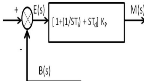
**Fig.4.** Block diagram of PID controller
