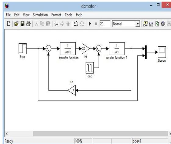
**Fig. 4.** Simulink model of S.E.DC motor
