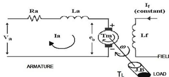
**Fig 2.** Circuit diagram of S.E.DC motor
