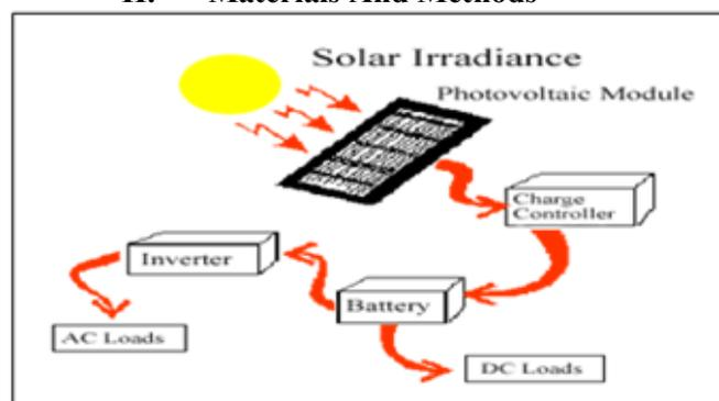
The Photovoltaic module (PV) or Solar panels are installed on the roofs, they convert the sunlight into the direct current(DC) power. The charge controller limits the rate at which the electric current is added or drawn from the electric batteries. The batteries being one of the main component of the solar power system, the
