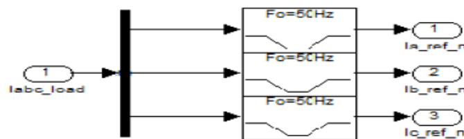
Fig (2) The band pass filter algorithm
