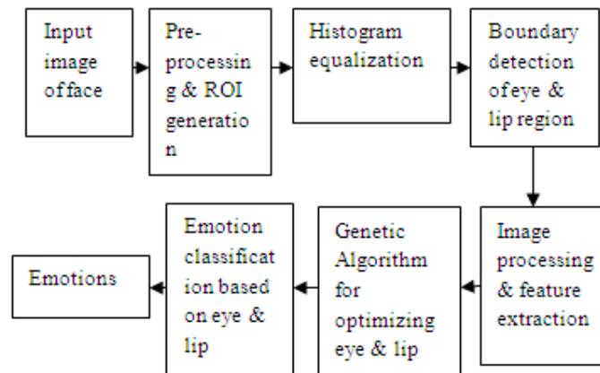
Fig.1. Block Diagram of Emotion Recognition Process
