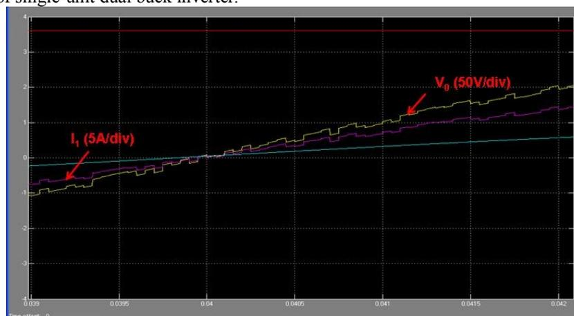
Fig. 6. Experimental result of single-unit half-bridge dual buck inverter at zero crossing period.
