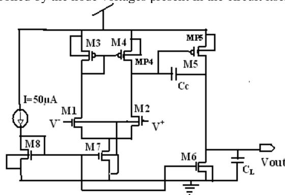
Figure.1. Two stage OPAMP with the compensation capacitor
