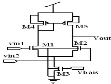
Figure 2. Differential amplifier circuit
