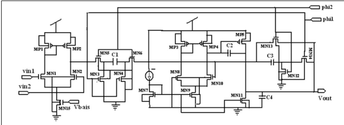
Figure 6: Schematic of humidity sensor with read out circuit
