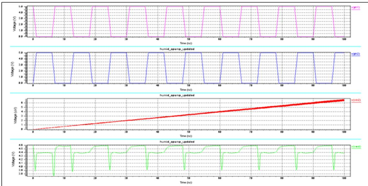
Figure 7: Waveform of humidity sensor with read out circuit
