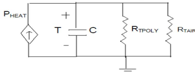
Fig 3: lumped element thermal circuit representing the self heating of a diode biased with constant current [4]
