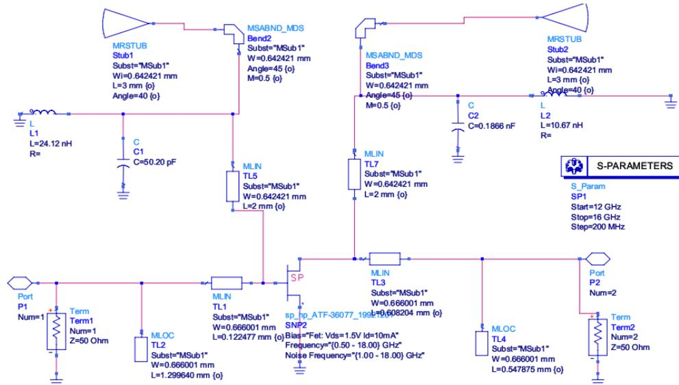
Fig. 4. LNA with distributed element in matching network and radial stub in biasing networks
