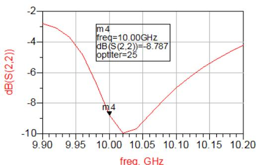
Fig. 11. Output reflection coefficient
