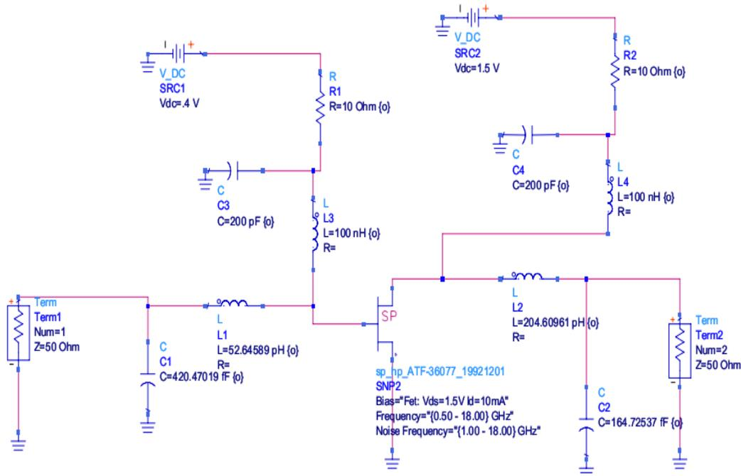
Fig. 2. LNA with lumped element in matching and biasing networks
