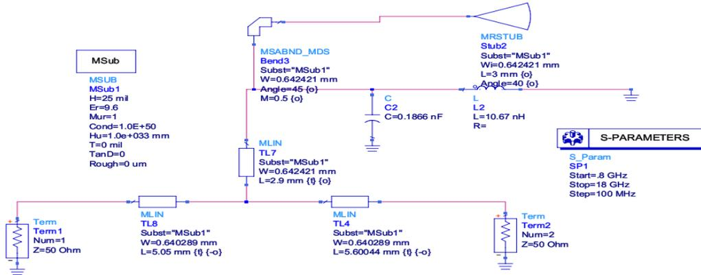
Fig. 5. Biasing network in ADS
