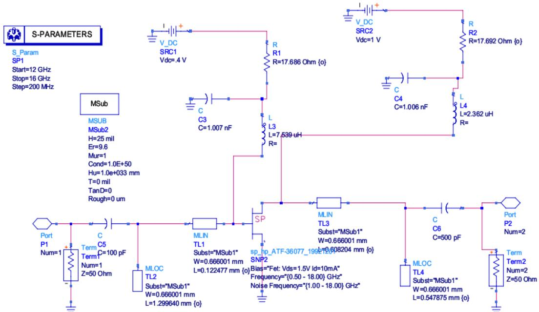
Fig. 3. LNA with distributed element in matching network and lumped element in biasing networks
