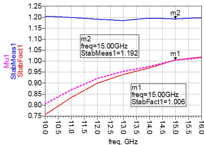
Fig. 1. Stability figure for active part of 15 GHz amplifier
