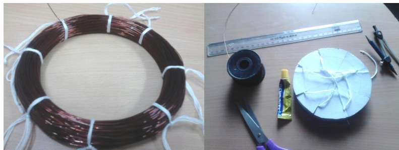
Figure 6: Magnetic coil and bobbin after construction.
