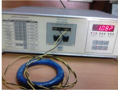
Figure 7: Testing of Coil using RLC Q-model 9410.
