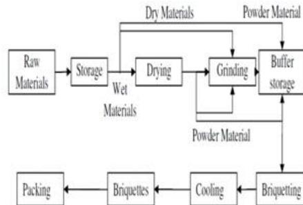
Figure 5.1 Flow diagram of biomass briquette production
