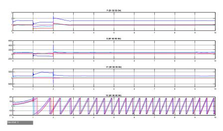
Fig. 7(c) Simulated wave-form for LLG fault without POD controller
