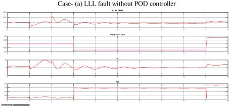
Fig.6 (a) Dynamic response of SSSC for LLL fault without POD controller
