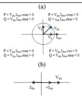
Fig. 4 SSSC phasor diagram
