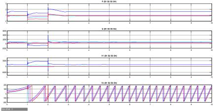
Fig. 7(d)Simulated wave-form for LLG fault with POD controller
