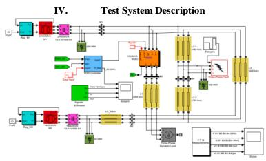
Fig. 5 Static Synchronous Series Compensator (SSSC) used for power oscillation damping
