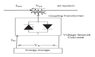
Fig. 3 Functional model of SSSC
