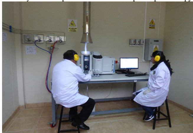
Figure no 2. Analysis of samples with atomic absorption spectroscopy equipment
