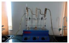
Fig.1 soxhlet method.
